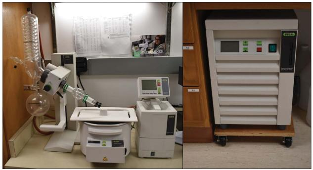
The **Rotavapor**<sup>®</sup> **R-100** is a high-quality rotary evaporator to meet the essential needs in classical laboratory applications. It is capable of a manually adjustable rotation speed of 20 to 280 rpm and equipped with an action jack lift for manual lifting of the evaporating flask. Included is the selected condenser, 1 L receiving and evaporating flasks and a vapor duct. It works in conjunction with the B-100 digitally controlled heating bath.
